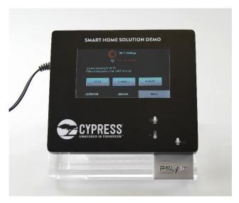
This touch demonstration device developed by Cypress includes a single layer PolyTC touch sensor from PolyIC
